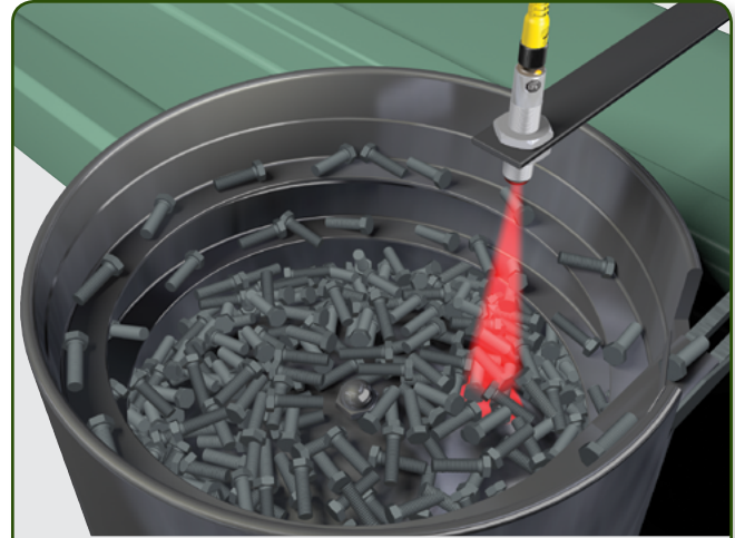
Feeder bowl application – A 42CM monitors bowl level to prevent component runoff. This background suppression model ignores reflections from the bowl to accurately detect the components only.
