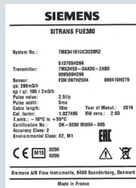
FUE380 transmitter label (with MID first verification)
